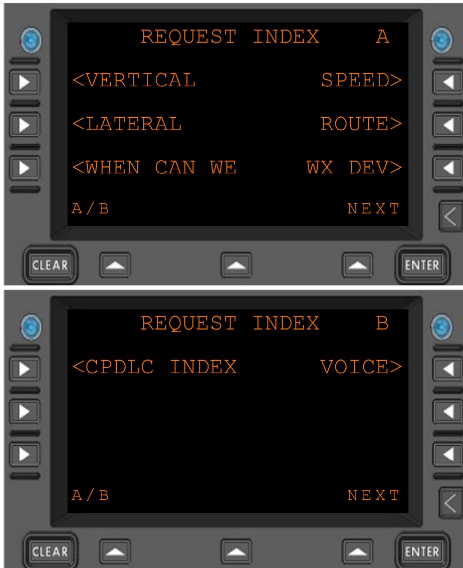
Figure 7.1.5-2 Request Index (Menu A and B), DO 280B
