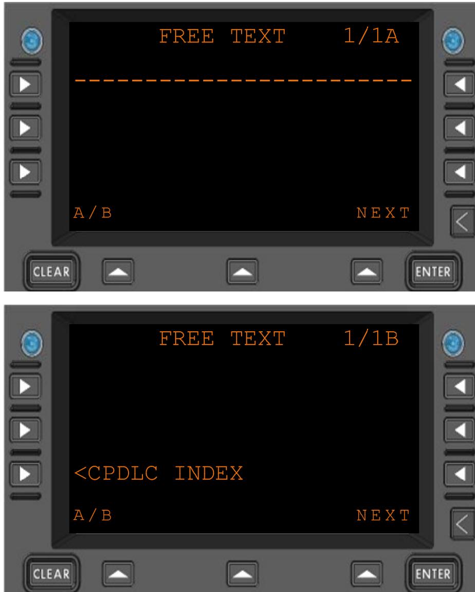
**Figure 7.1.2-1 CPDLC Free Text Menu (Menus A and B)**
